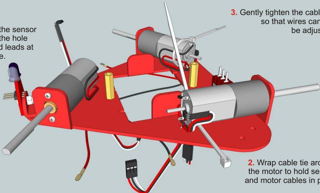
2. Wrap cable tie around the motor to hold sensor and motor cables in place.
